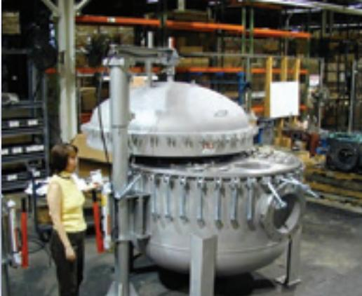
Eaton MAXILINE bag filter vessels are designed for flow rates to 4400 gallons per minute—excellent for pre-filtration protection of membrane systems, mixed bed resin systems, etc., available in 3 - 36 bag configurations. Bag filter elements are available in nominal and absolute ratings, pleated and non-pleated; 1 micron and above.
