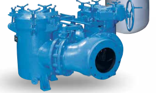
Model 52 synchronized butterfly valves minimize the effort of switching flow from one basket chamber to the other.
