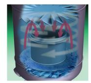
Vortex Containment Plate (VCP) prevents re-entrainment of separated liquid.
