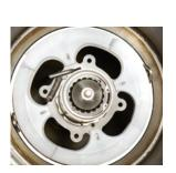
Eaton's unique spring loaded cleaning disc (shown here in an MCS-500) ensures intimate contact with the filtration screen to thoroughly and uniformly clean the media.
